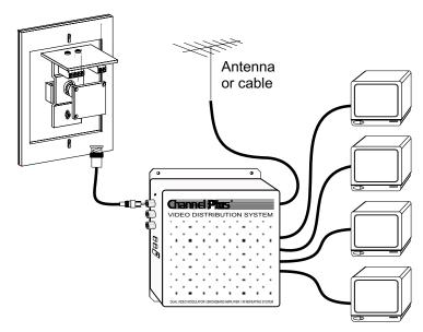
Using an All in One Video Distribution System such as a ChannelPlus model 3015, you may view the camera on an unused UHF or cable channel. (For example, the front door camera could be UHF channel 50. All antenna channels will appear normally.)
